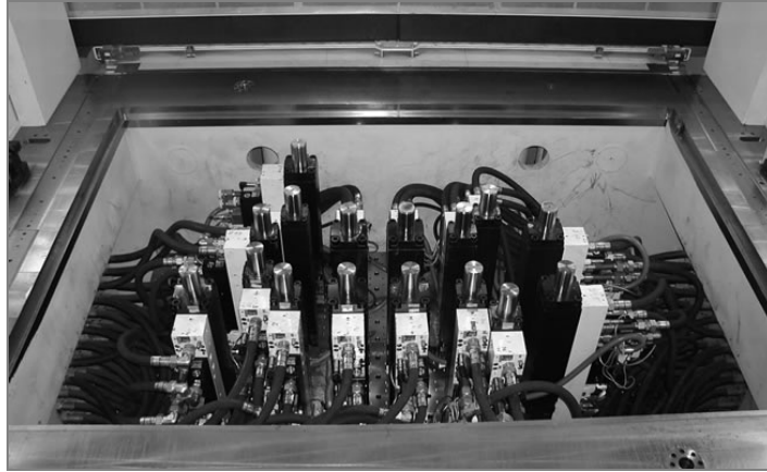
Fig. 10. Multi-point cushion (16 axes)
