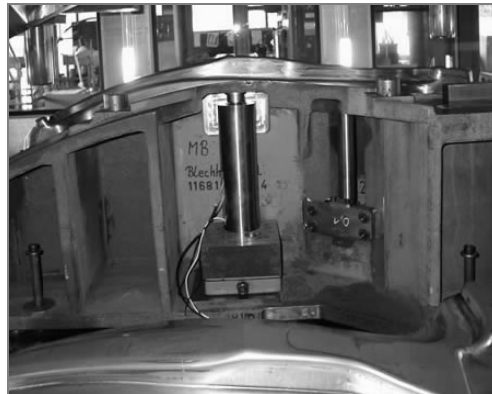
Fig. 12. Piezo actuator built into the tool (B pillar)
