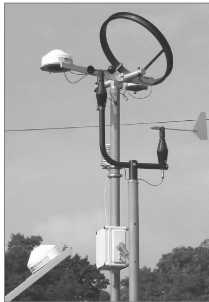
Fig. 1. Actinometric station in SolarLAB Photovoltaic Laboratory in Wrocław
