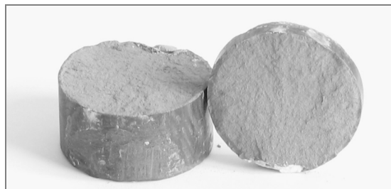
Fig. 3. Compact made of Ti6Al4V titanium alloy powder produced by GA, after compaction under pressure of 1019 MPa
