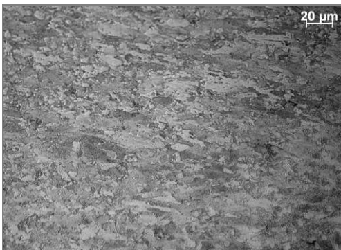
Fig. 9. Metadynamically recrystallized structure of steel solution heat-treated from 1000 °C after 40% deformation and isothermal holding for 4 s
