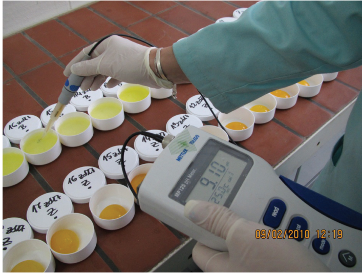
Fig. 3. Measurement of the hydrogen ion concentration in egg albumen and yolk
