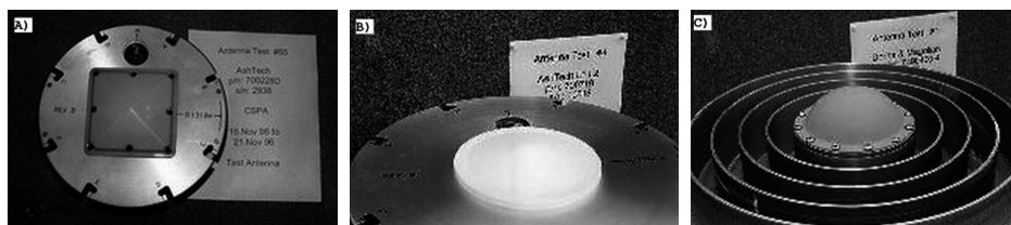
Fig. 5. Antenna used in measurements: A) ASH700228A; B) ASH700718A; C) AOAD_M_T (source: http://www.ngs.noaa.gov/ANTCAL/ )
