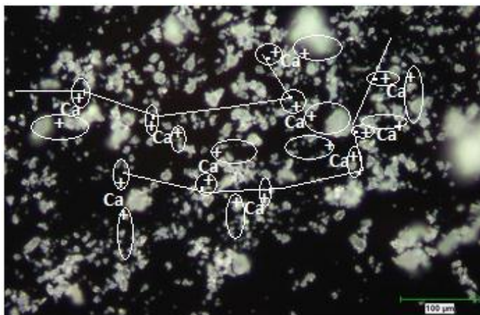
Fig. 7. Schematic illustration of \text{Ca}^{2+} activation on adsorption of high molecular weight anionic flocculant onto a negatively charged suspended travertine fines
