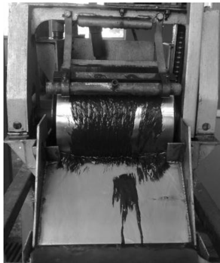
Fig. 2. Laboratory size low intensity drum type wet magnetic separator
