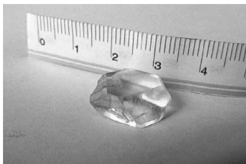
Fig. 2. A photograph of a grown \text{NaNH}_4\text{SeO}_4 \cdot 2\text{H}_2\text{O} single crystal doped with \text{Cr}^{3+}
