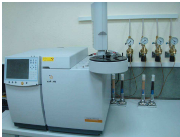
Fig. 3.37 View and operation diagram of a gas chromatographer [5]
