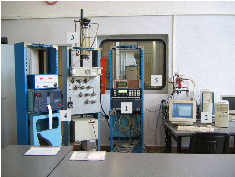
Fig. 3.2 A control room for engine test stand
