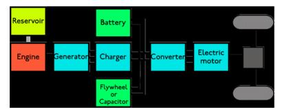
Figure 1.2. Structure of a series hybrid vehicle with flywheel or ultracaps as peak power unit [1],[8],[29],[35].
