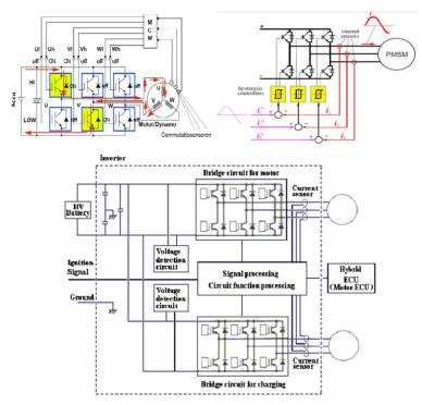
Figure 4.1.21. The inverter supplying motor/generator of Honda Civic IMA (above left) with detailed of control of brushless motor current (above right), control unit with inverters supplying motor and generator in TOYOTA Prius III (bellow) [29],[35].
