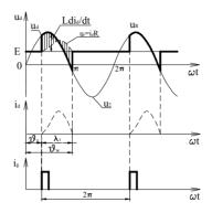
Figure 3.2.5. The waveform of DC voltage, current and gate impulse for RLE-load [3],[4],[5],[11].
