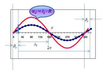
Figure 3.2.3.Explanation of angle of ignition  $\mathcal{G}_z$  and angle of conduction  $\lambda_T$ .
