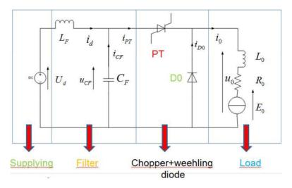
Figure 3.2.16.Basic structure of the SRC choppers [4].
