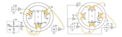
Figure 4.1.11. The Hall effect sensors commutation of  $3-\varphi$  brushless motor (left) and  $2-\varphi$  pushpull drive (right) [7],[8],[33],[35].
