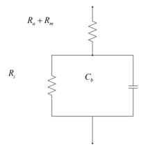
Figure 2.1.2. The equivalent circuit for an energy cell [1],[36],[37].
