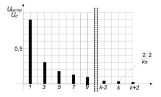
Figure 3.2.31.Spectrum of harmonics derived from Fourier analysis [3],[4],[5],[11]...
