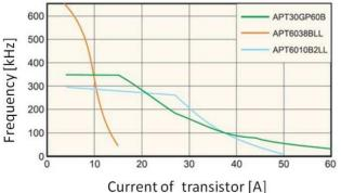
Figure 3.1.13.The catalogue characteristics of transistor [A] APT6010B2LL and IGBT APT30GP60B
