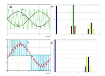
Figure 3.2.36. The waveform of output voltage and output current of the inverter a) and spectrum voltage for two switches b) and four switches [3],[4],[5],[11].
