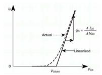
Figure 3.1.9. The transfer characteristic of MOSFET [3],[5],[8].
