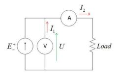
Accurate measurement of current value
