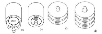
Figure 4.1.10. The cylindrical construction: (a) outside rotor, (b) inside rotor and Pancake motor construction: (a) single stator, (b) double stator [33],[35],[48].
