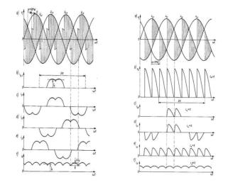
Figure 3.2.13. The waveform of DC voltage and current for continues mode (left) and impulse mode (right), including commutation process [3], [4], [5], [11].a) DC voltage output waveform b), c), d),e) phase supplying current of rectifier f) DC output current waveform
