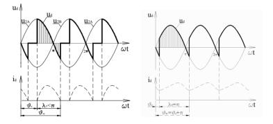
Figure 3.2.8. The waveform of DC voltage and current for RL-load for two pulse rectifier the impulse status (left) and continues one (right) respectively[3],[4],[5],[11].
