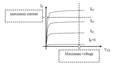
Figure 3.1.4.Output characteristic of a BJT [3],[5],[8].
