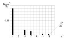
Figure 3.2.33. Spectrum of output voltage for of three phase inverter with connected neutral point [3],[4],[5],[11].
