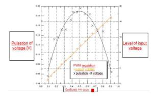
Figure 3.2.20. The characteristic of output voltage and pulsation of voltage at PWM.
