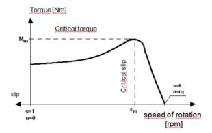
Figure 4.1.6. Torque versus speed [8].
