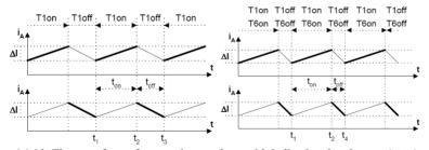
Figure 4.1.19. The waveform of current in one phase with indication the time on ( $t_{on}$ ) and the time off ( $t_{off}$ ) for unipolar (left) and (bipolar) mode of control [6],[7],[8],[33],[35].
