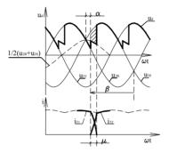
Figure 3.2.11. The waveforms of DC voltage and current for R-load when include of the commutation process [3],[4],[5],[11].
