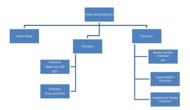
Figure 3.1.1.The semiconductors typically used in power electronics.
