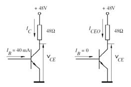
Figure 3.1.6. BJT switched on (left) and switched off (right)
