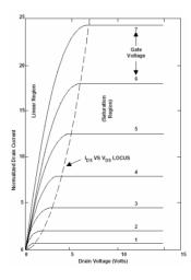
Figure 3.1.8. Output characteristic (current vs voltage) for example [3],[5],[8].
