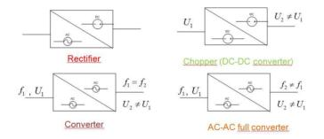
Figure 3.2.1. Family of solid state power converters categorized according to their function.
