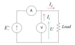
Accurate measurement of voltage value
