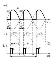
Figure 3.2.7. The waveform of DC voltage, current and gate impulse for R-load when used the two pulse rectifier [3],[4],[5],[11].
