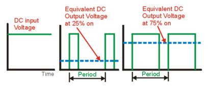
Figure 3.2.17. Principle of controlling of output voltage of choppers [3], [4], [5], [11].
