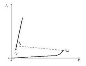
Figure 3.1.15. The characteristics of work of thyristor. [3], [5], [8].
