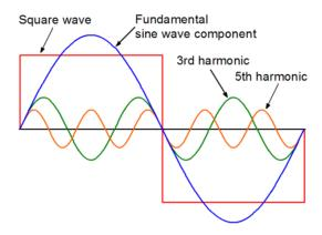
Figure 3.2.30.Square wave voltage with fundamental, 3th and 5th harmonics respectively[3],[4],[5],[11].
