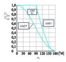
Figure 3.2.14. The characteristics of control of six pulse rectifier [3],[4],[5],[11].
