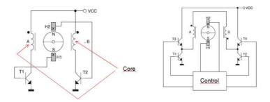
Figure 4.1.13.The main circuits of control BLCD machines: unipolar (left) and bipolar (right) [7],[8],[33],[35].
