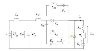
Figure 3.2.21. The circuit of chopper with parallel circuit of commutation.
