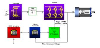
Figure 4.1.8. Three-phase AC induction motor driven by a power converter [31].
