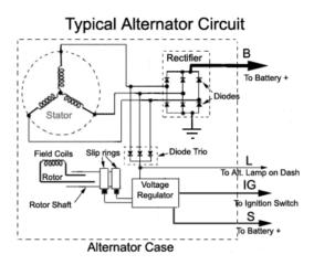
Figure 3.2.15.The six pulse rectifier transfer AC alternator voltage to the DC battery and/or to another units voltage with three pulse rectifier for voltage regulator.
