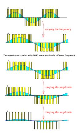
Figure 3.2.37. The idea of amplitude and frequency variation [3], [4], [5], [11].
