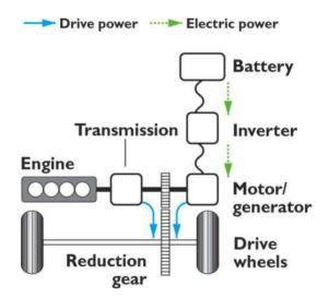
Figure 1.4. Structure of a parallel hybrid electric vehicle [1],[8],[29],[35].
