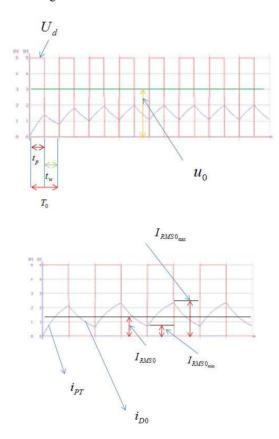
Figure 3.2.18. Waveforms of voltage and current of the choppers [3],[4],[5],[11].
