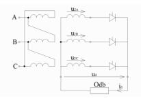
Figure 3.2.10. The three pulse rectifier as the bridge variant [3],[4],[5],[11].
