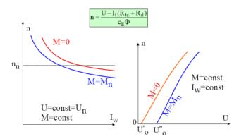
Figure 4.1.5.Control characteristics of the DC motors [12].
