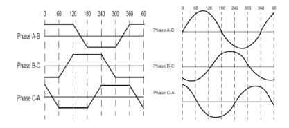
Figure 4.1.9.The electromotive force for the BLCD trapezoidal (left) and sinusoidal (right) [7],[8],[33],[35].
