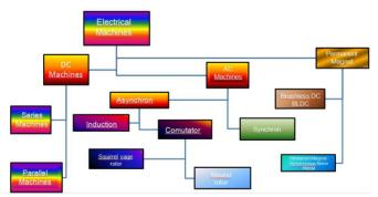
Figure 4.1.Various types of electrical machine used in hybrid and electrical vehicles.
