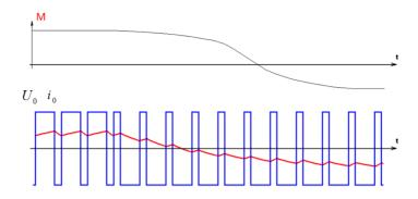
Figure 3.2.25.Transient from quadrant 1 to quadrant 3 via quadrant 2[3],[4],[5],[11].
