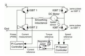
Figure 3.2.26. The servomotor control circuit [29].
