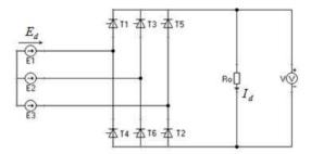
Figure 3.2.12. The six pulse bridge rectifier variant [3],[4],[5],[11].
