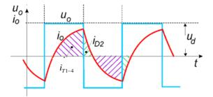
Figure 3.2.29. Waveform of output voltage of the inverter respectively [3], [4], [5], [11].
