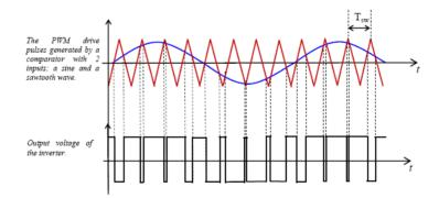
Figure 3.2.35.Idea of control of PWM inverter [3],[4],[5],[11].
