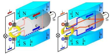
Figure 4.1.1. The model of conventional DC parallel motor with two and four sectors [12].
