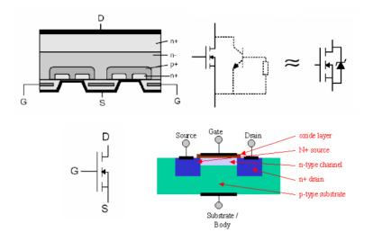
Figure 3.1.7. Simplified structure and circuit symbols of a n-channel MOSFET[3],[5],[8].
