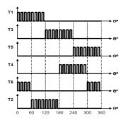
Figure 4.1.17. Sequence of control of bipolar status switching of valve .[6],[7],[8],[33],[35].
