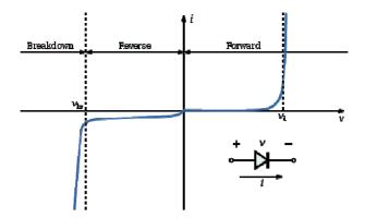
Figure 3.1.2. The characteristics of a P-N junction diode (not to scale) [3],[5],[8].
