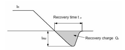
Figure 3.1.3.Current during blocking of a power diode [3],[5],[8].
