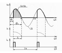
Figure 3.2.3. The waveform of DC voltage, current and gate pulse for R-load [3],[4],[5],[11].
