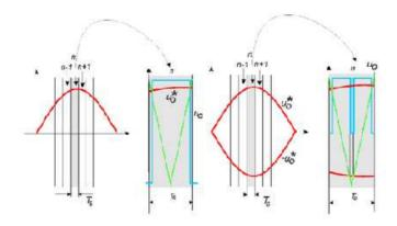
Figure 3.2.34.Idea of approximation of the sinus form of output voltage by using of a very high frequency of switch on-off (left for two transistor and right for four transistor bridge) respectively [3],[4],[5],[11].
