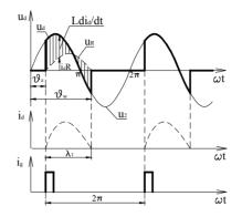
Figure 3.2.4. The waveform of DC voltage, current and gate impulse for RL-load [3],[4],[5],[11].
