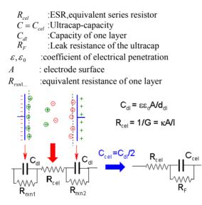
Figure 2.2.4. Ultracapacitor equivalent circuit [1],[8].
