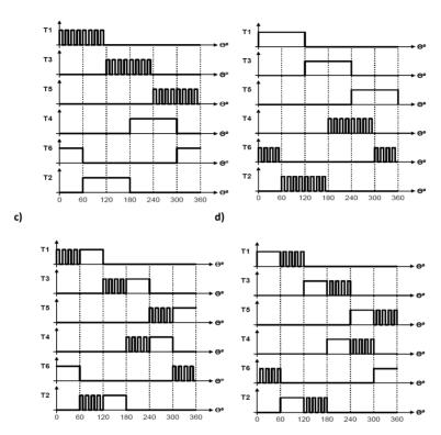
Figure 4.1.17. The sequence of control of unipolar status switching of valve a) C120Q+ sequence, b) C120Q- sequence, c) C60Q+ sequence, d) C60Q- sequence [6],[7],[8],[33],[35].
