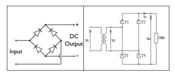
Figure 3.2.6. The two pulse rectifier Graetz (left) and bridge (right) circuits. [3],[5],[8].
