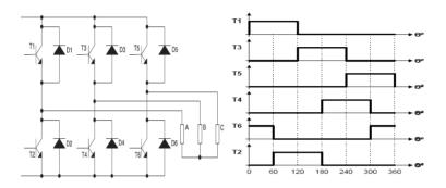
Figure 4.1.16. The six pulse full bridge (left) and general sequence of switching of transistor (right) [6],[7],[8],[33],[35].
