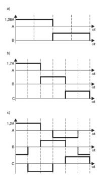
Figure 4.1.14.The current waveform a)two phase unipolar, b)three phase unipolar, c)three phase bipolar [6],[7],[8],[33],[35].
