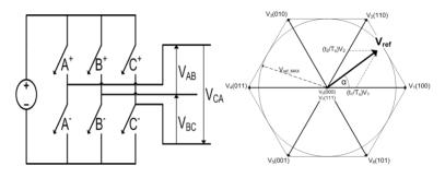
Figure 3.2.38. The method of space vector modulation [3], [4], [5], [11].
