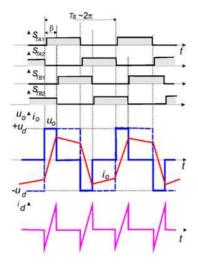
Figure 3.2.32. Waveforms of output voltage and current for the single-phase voltage source inverter [3],[4],[5],[11].
