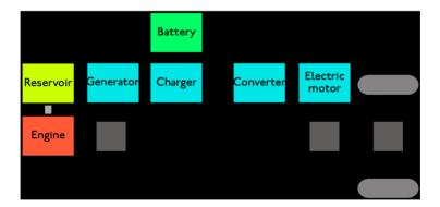
Figure 1.6. Simplified structure of a combined hybrid electric vehicle [1],[8],[29],[35].
