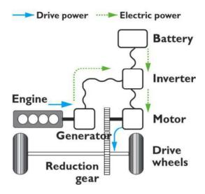
Figure 1.1. Structure of a series hybrid vehicle [1],[8],[29],[35].
