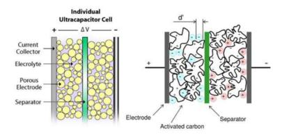
THE ULTRACAP=supercap=Electrochemical Double Layer Capacitor EDLC
