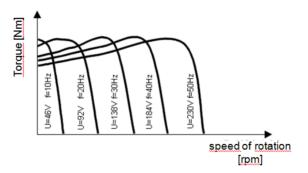
Figure 4.1.7. Family of torque characteristics versus speed [8].
