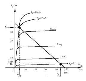
Figure 3.1.5.Output characteristic of a BJT with triangle of save power [3],[5],[8].
