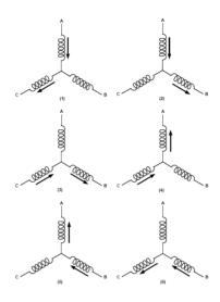
Figure 4.1.15. The winding energizing sequence with respect to the hall sensor [7],[8],[33],[35].
