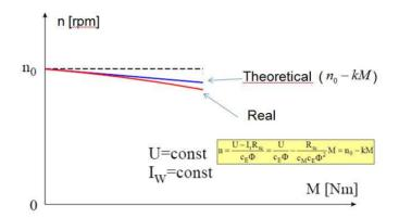
Figure 4.1.4. Mechanical characteristics of the DC parallel shunt motor [12].
