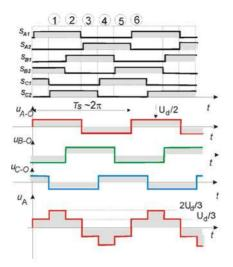
Figure 3.2.33. Square waveform of voltage of the three phase inverter [3],[4],[5],[11].
