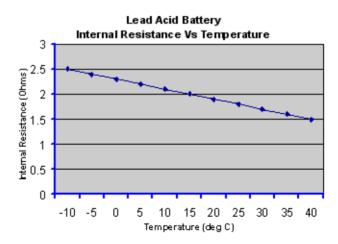
Figure 2.1.3. The influence of temperature on internal resistance of battery[1],[8],[36],[37]. .
