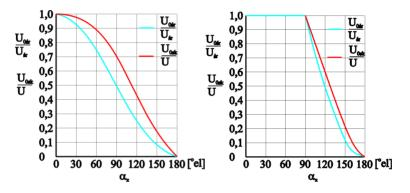
Figure 3.2.9. Characteristics of control of two pulse rectifier for R-load (left) and RL-load (right) [3],[4],[5],[11].
