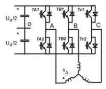
Figure 3.2.33. The circuit of the three phase inverter [3], [4], [5], [11].
