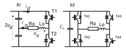
Figure 3.2.28. The single-phase voltage source inverter a) based on two transistors b) based on four transistors respectively [3],[4],[5],[11].
