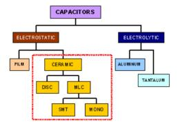
Figure 2.2.1 Classification of conventional capacitors [8],[19],[20].
