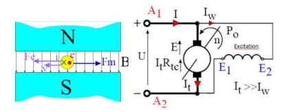
Figure 4.1.3.The phenomena in the space of magnet N-S with equivalent circuit of parallel shunt DC motor (right) [12].
