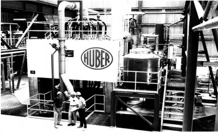
Fig. 8. View of the superconducting HGMS built by Eriez Magnetics, Erie, PA, USA and installed at the plant of J.M. Huber where it has been on line since 8 May 1986 (Watson, 1994).
