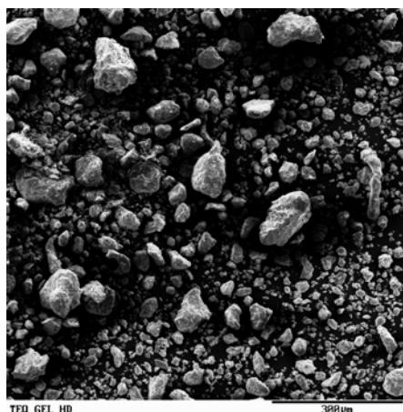
Fig. 2. Teqgel HD bentonite (a) multimodal particle size distribution (b) SEM micrograph.
