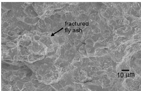
Fig. 7. The tensile fractured surface of the composite
