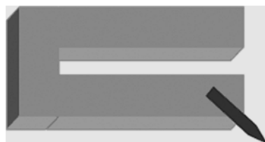
Fig. 4. Schematic picture showing a tip mounted to a normal tuning fork
