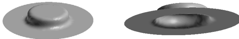
Fig. 14. Different views of the simulated drawn cup with the initial blank size of 180 mm
