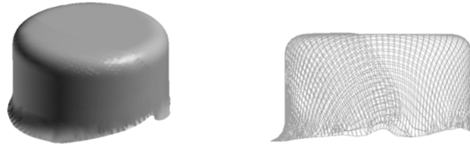
Fig. 5. Different views of a simulated drawn cup with an initial tailored blank size of 140 mm
