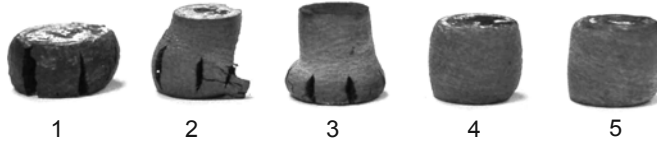
Fig. 1. Specimens surface appearance after compression test
