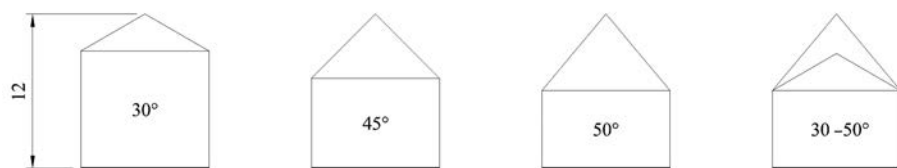
Fig. 4. Examples of different roof slopes according to record of the local plan of Biestrzyków
