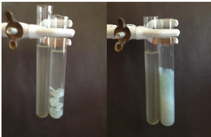
Fig. 4. Addition of NaOH to filtered pulp sample (pH 5.5)
