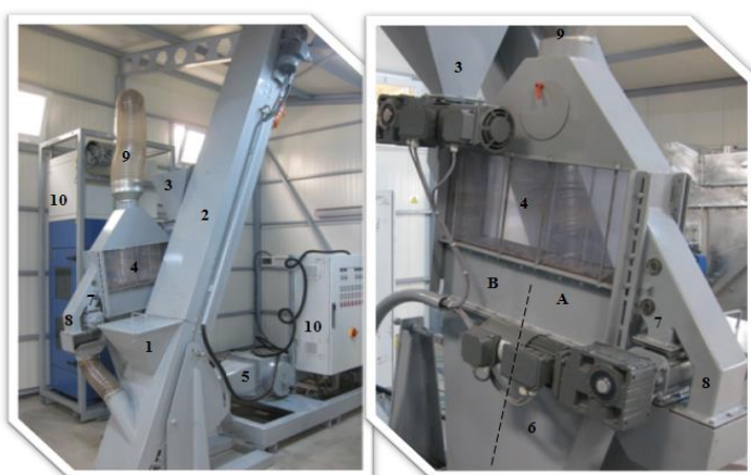
Fig. 1. Lab scale Allair stratification jig facility (1-feed chute, 2-belt conveyor, 3-feed chute, 4-jigging cell, 5-pulsed air production and distribution mechanism, 6-fluidized air tank, 7-dense particle discharge channel, 8-light particles discharge, 9-ventilation pipe, 10-filter unit)
