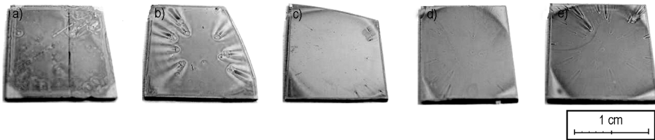
Fig. 1. Thin layers of spin-on dielectrics (HSQ polymer) coated at various rotational speeds: a) 1000 rpm, b) 2000 rpm, c) 3000 rpm, d) 4000 rpm, e) 5000 rpm
