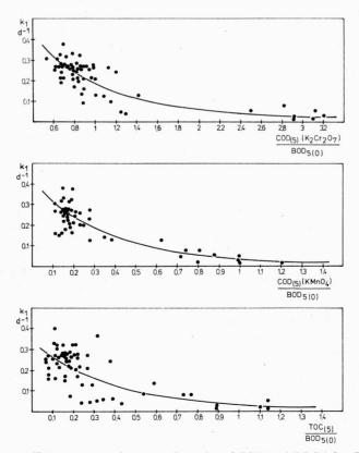
Fig. 6. Reaction rate coefficient constant  $k_1$  versus the ratios of COD and TOC (after five days of aeration) to BOD<sub>5</sub> (non-treated samples)
