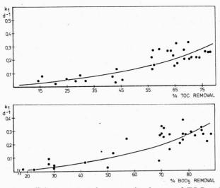
Fig. 5. Reaction rate coefficient constant  $k_1$  versus the degrees of TOC and BOD<sub>5</sub> removals
