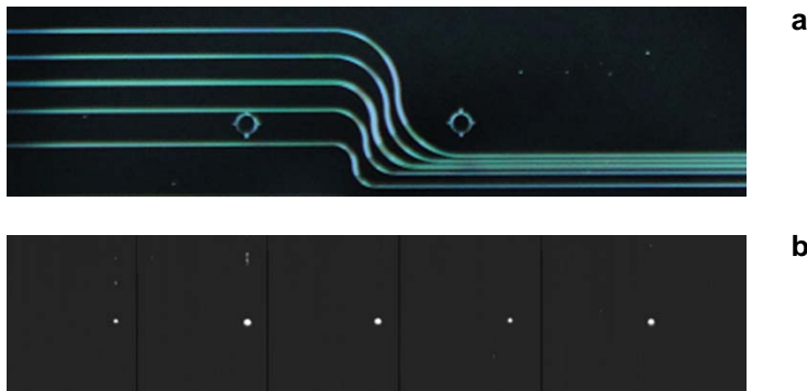
Fig. 5. Device of S-bend composed of two 90^\circ waveguides (a); near-infrared field of the device of S-bend (b).
