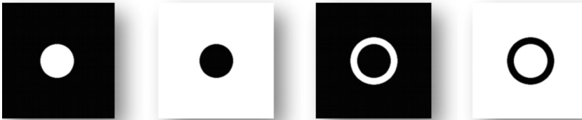
Fig. 2. Basic spatial filters (left to right): low-pass (LPF), high-pass (HPF), band-pass (BPF), band-stop (BSF).
