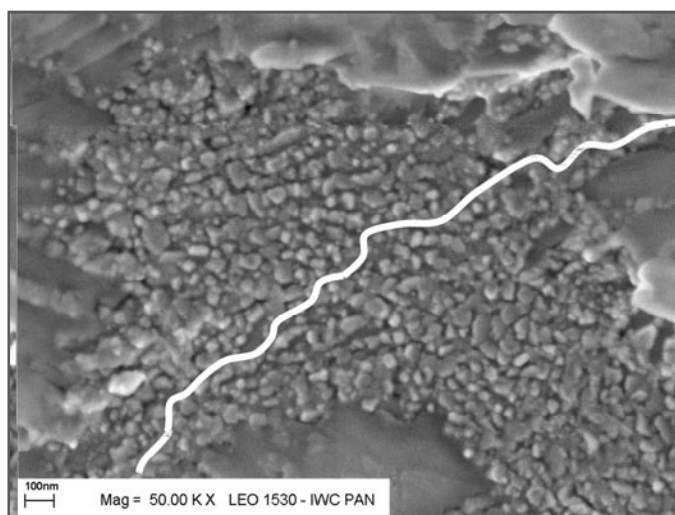
Fig. 6. Scanning electron microscopy (SEM) micrograph of the sample described by x = 0 after annealing at T_{0c} = 540 °C. The white line between nanocrystallites depicts an easy conduction path
