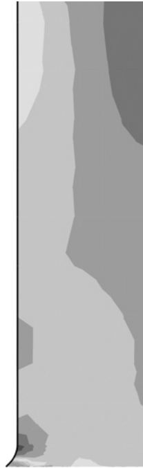
Fig. 3. Axial stress counter in the insert (MPa)
