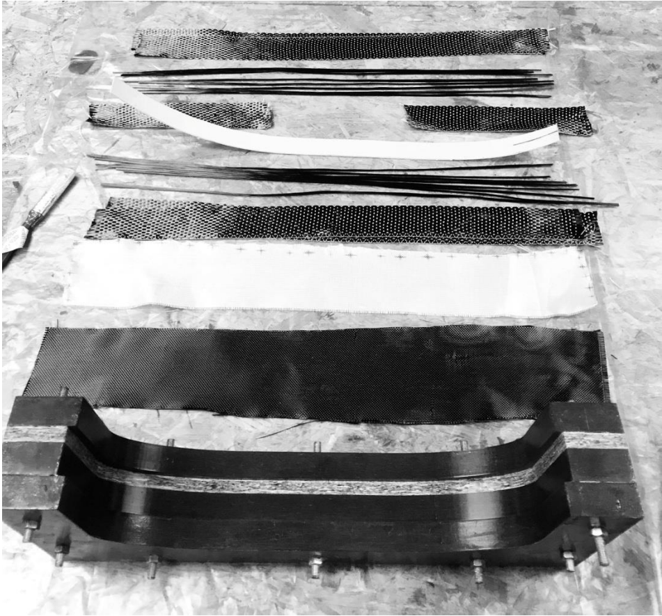
Fig. 1. This picture shows mold (the first one from the bottom) and materials in order they are used starting from the bottom of the picture.
