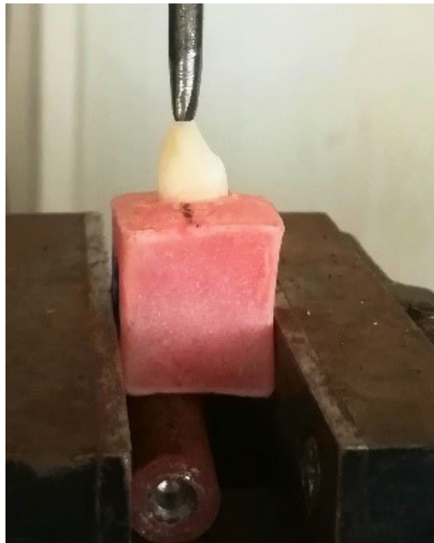
Fig. 2. Load applied at the incisal edge using the Instron testing machine
