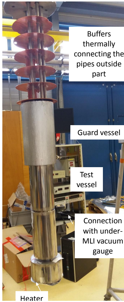
Figure 24: Test cryostat picture: the test vessel is a cylinder measuring 0.5 m with an external surface of 0.2 m 2
