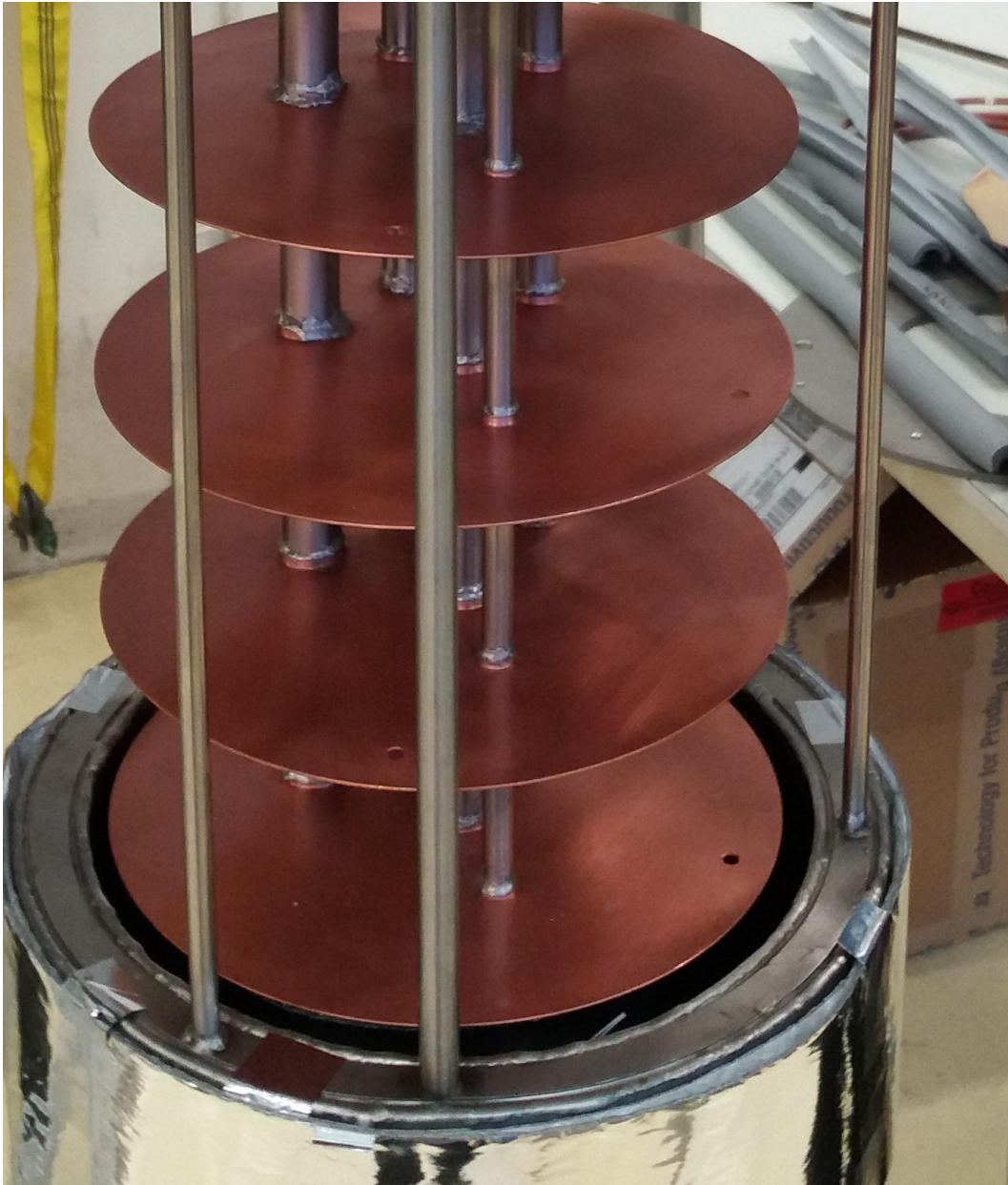
Figure 25: Buffer thermal shield welded on pipes, liquid Nitrogen annular vessel
