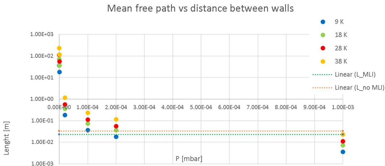
Figure 63: Free mean path for different residual pressure levels and mean temperatures between walls
